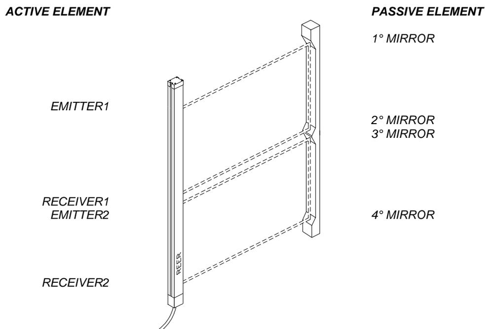
**Figure 2 - MI TRX / J TRX with 3 beams**
