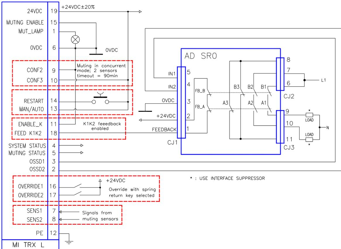
**EXAMPLE OF CONNECTION : J TRX L WITH AD SR0 WITH START/RESTART INTERLOCK ACTIVATED**
