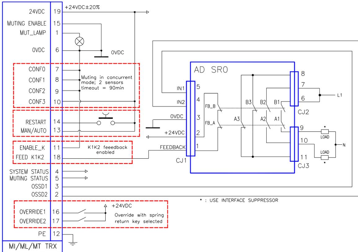
**EXAMPLE OF CONNECTION: MI TRX L WITH AD SRO WITH START/RESTART INTERLOCK ACTIVATED**
