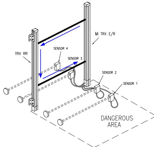
**Figure 7 - Connection with 4 external sensors**
