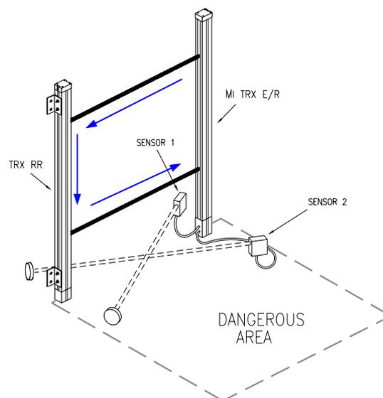
**Figure 4 - connection with 2 external sensors**
